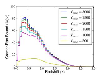
FIG. 6. The super tomographic Cramer-Rao bound on the lensing kernel with different  $\ell$ -cuts. Information is primarily lost intermediate redshifts, near z=0.5, and catastrophically lost below  $\ell_{max}<1000$ .
